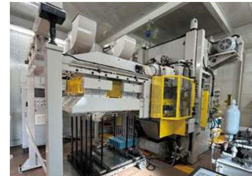
Introduction of new fin press line for WA coils
