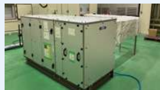
Cooling capacity test of air handling unit in comprehensive testing facility
