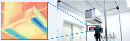
Dew condensation test of fan coil unit in variable temperature and humidity room
